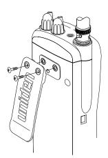
Do not tighten the screws too tight. You can damage the case or clip.
